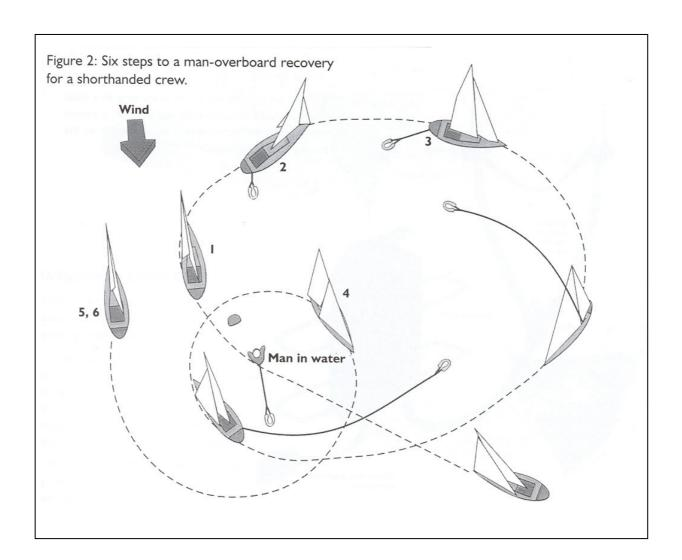
2. The Lifesling is deployed by opening the bag on the stern pulpit and dropping the sling into the water. It will trail astern and draw out the line.
